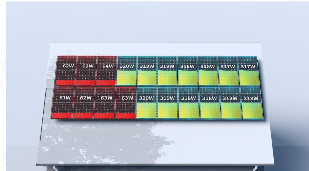
Shadow occlusion of traditional string system
